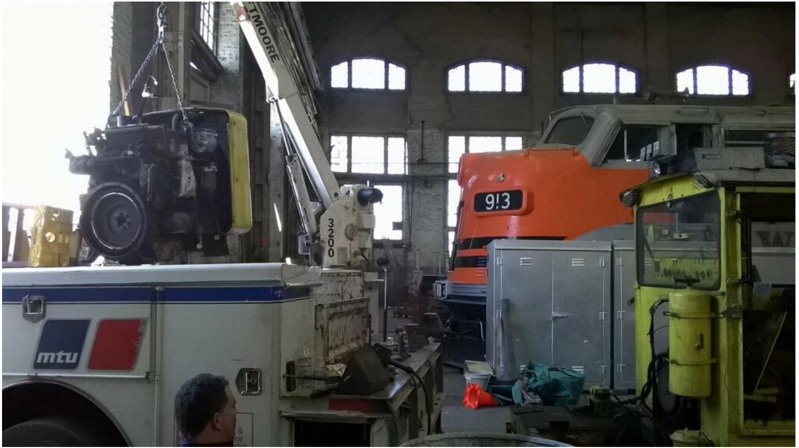
On Wednesday, the 60-year old (plus) 3-53 Detroit Diesel engine was hoisted out of the Kalamazoo
