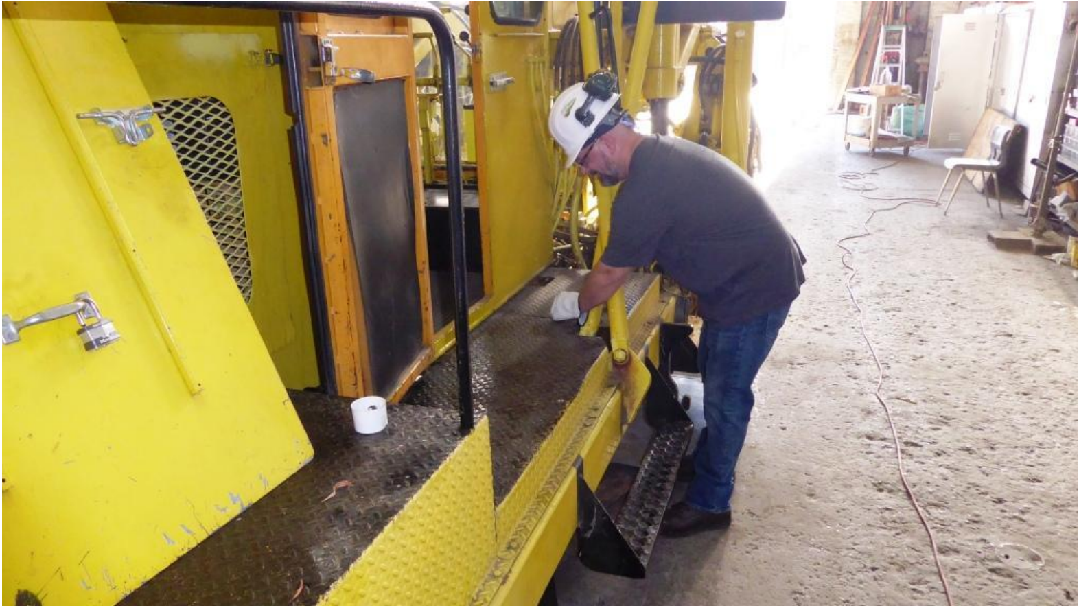
DJ removes the deck-plates over the brakes of the tamper
